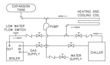
FIG. 41 Installation with a Chilled Water System
